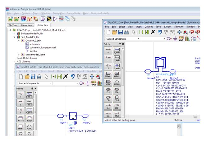
For simulations where you use this cell, you can now use ADS feature Dynamic Model Selection to choose between the S-parameter and equivalent circuit model views with:
