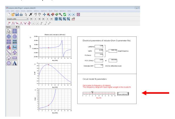
On the bottom right side, you see a frequency slider. Select your frequency of interest, i.e. the operating frequency where you want best accuracy for your extracted model. This frequency will be used to extract initial values for the equivalent circuit mode fit.
