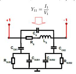
InductorModelFit comes with equations to calculate both single ended and differential results from the 2-port configuration shown above. You do not need to assign differential ports in the ADS simulations. The differential results are obtained by calculation in the data display.
