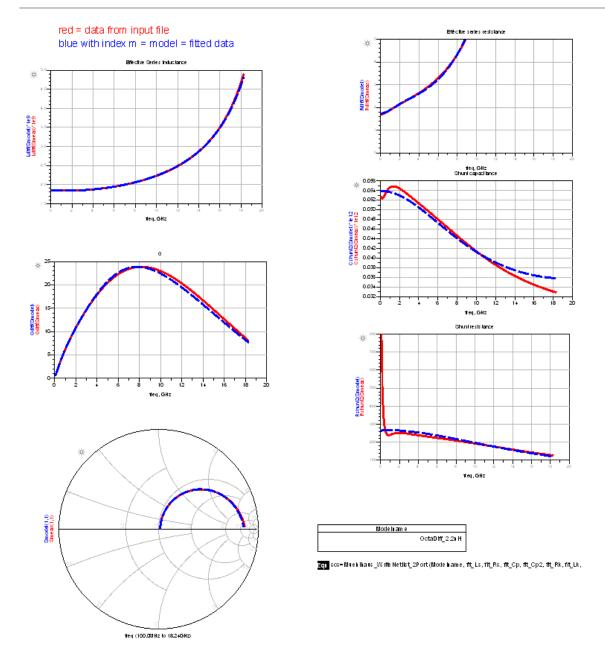
Plots show the comparison for differential L,Q,R and shunt capacitance and shunt esistance and single ended S11. The data display is configured to automatically write an \*.scs netlist for Spectre to the same directory where the S-parameter file is located.
