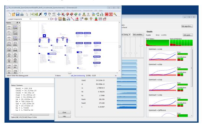
When the optimization has finished, close the optimizer cockpit and update the schematic with the optimized values<sup>3</sup>.
