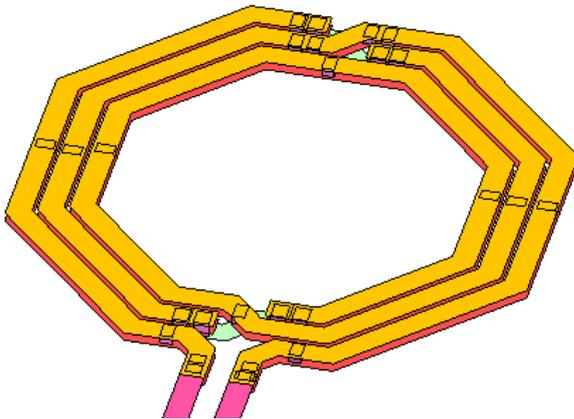
The reason for not changing the via properties is that the current will "see" the true physical via properties in those places where current flows, and we should not try to combine the total cross section of the entire big via array into some effective properties for the remaining vias. Don't worry if this thought is confusing here - we will come back to this later when we discuss Sonnet via merging and via meshing.
