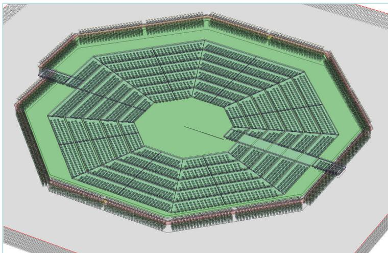
We will investigate modelling techniques that address this problem, to reduce simulation time and memory requirement. These techniques are based on the analysis via array behaviour at RF frequencies, which leads to possible via simplification.
