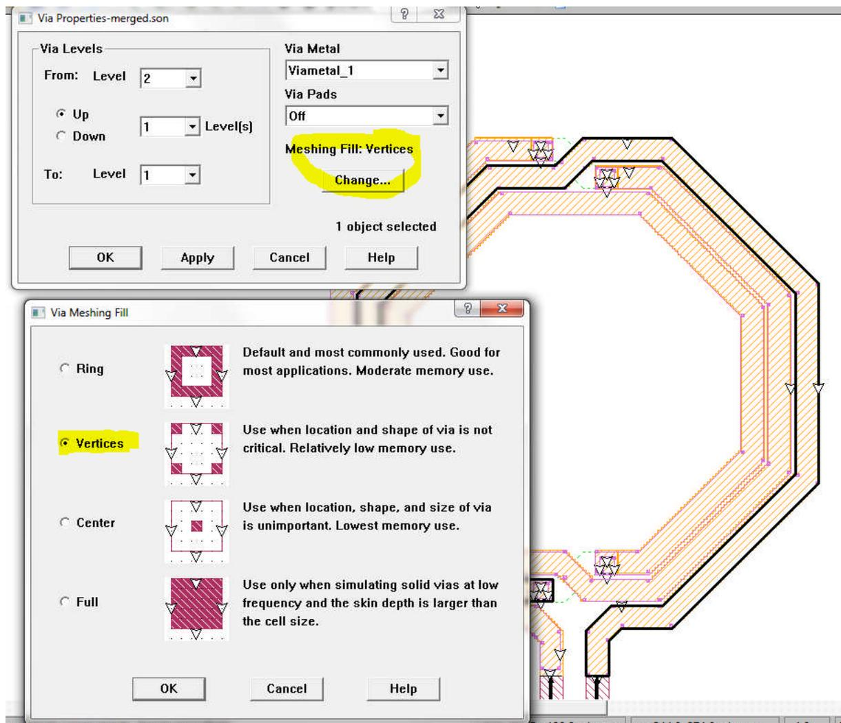
The effect is that the number of via subsections is reduced, and that they are only in a few places. With via subsections only in a few places, conformal mesh can be used in large parts of the model.
