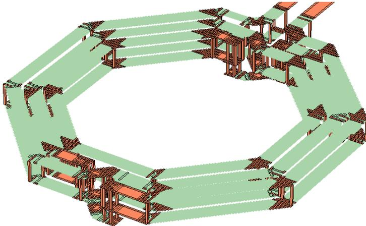
Conformal mesh is kept intact for most of the model, and automatically reverts to staircase only near the via subsections<sup>2</sup>.
