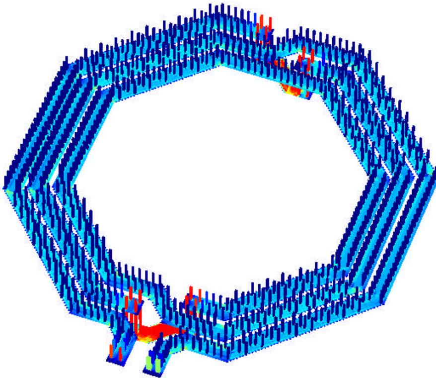
Red indicates high current and dark blue indicates no current. As you can see, even at this low frequency of 0.1 GHz, the current flows mostly through the vias at the "end" of the line, where the current has to split to the parallel conductors. In between, there is very small current. Once the current has split onto the parallel conductors, it just keeps flowing in parallel, without changing the layer, until it reaches the vias at the end of the parallel line.
