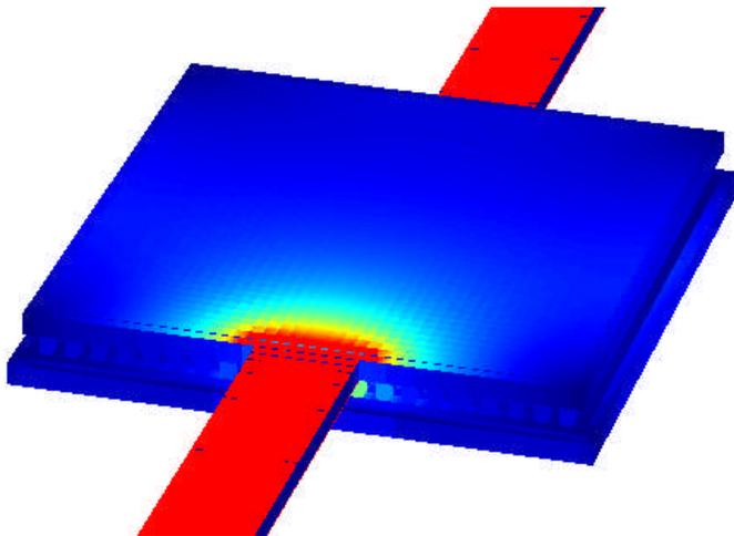
The topic of this application note is inductors, not MIM, but we can learn something useful from these pictures: the vias in an array are not of equal importance. The edge vias are most important, whereas the inner vias have only small RF current. This means that we can selectively remove vias, with very little change in results.
